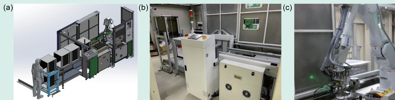
Fig. 2: (a) Schematic drawing of the automatic sample loading/unloading system. (b,c) Photographs of the automatic sample loading/unloading system.
